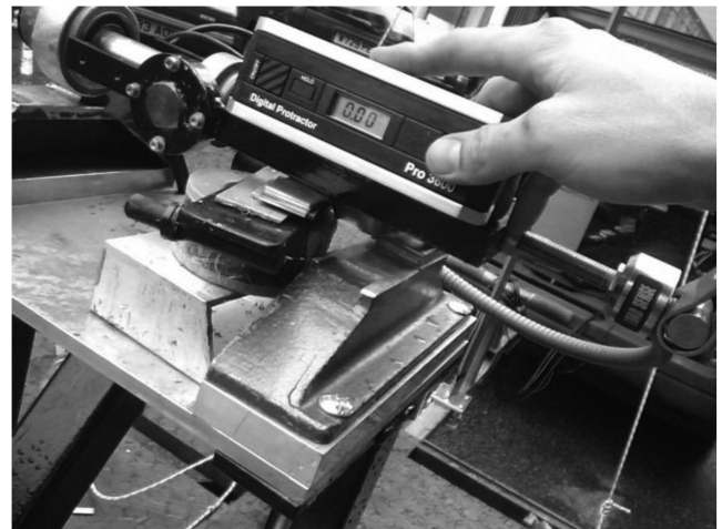
Fig. A1 A digital inclinometer is used to set the angle of the arm during calibration.
