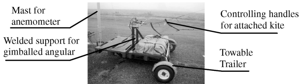
Fig. 9 The dynamometer and the attached kite.
